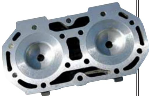
Jet World decked the stock head (left) to increase compression, while it also modified the carbs (right) from 38mm to 40mm to improve flow.
