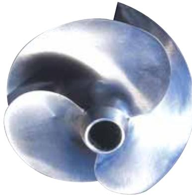
(Right) Skat-Trak's 13/18° impeller helped complement the added low-end power provided by this package. (Far right) Advent's Ignition replaces the stock component to advance timing at low rpm for improved acceleration and backs off at high rpm to reduce detonation.
